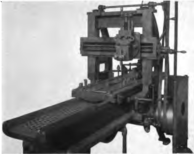
Fig. 1. Planer-Bed enclosed, to eliminate Danger from the Reciprocating Table.* Note also Belt Guard.
